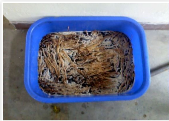
FIGURE 3 Surface modification of habara fiber
