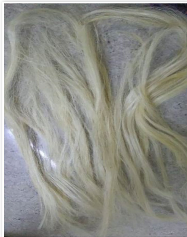
FIGURE 2 Extracted habara fiber
